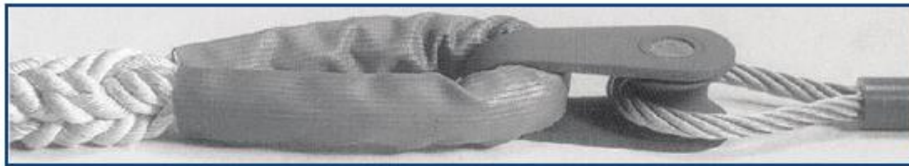
b) Wire rope in the sheave, fibre rope around the body. Mandal
