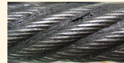
Left-hand ordinary lay (LHOL) wire rope (close-up). Right-hand lay strands are laid into a left-hand lay rope.
